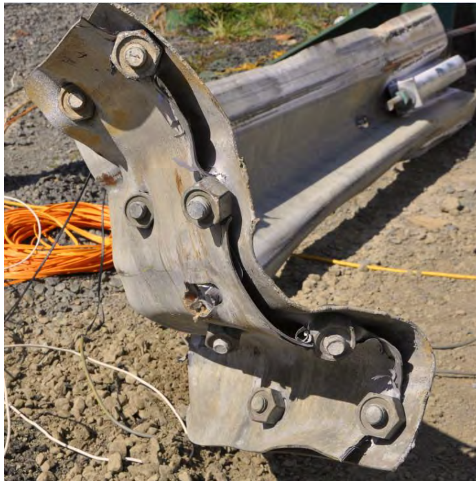
Figure 353. Results of Test 14004F with rail tear passing through all four downstream splice-bolt holes.
