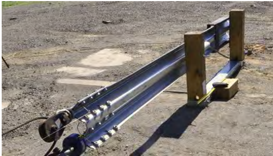
Figure 316. Pre-test photo of Test 14001I for 2" slack-cable case.
