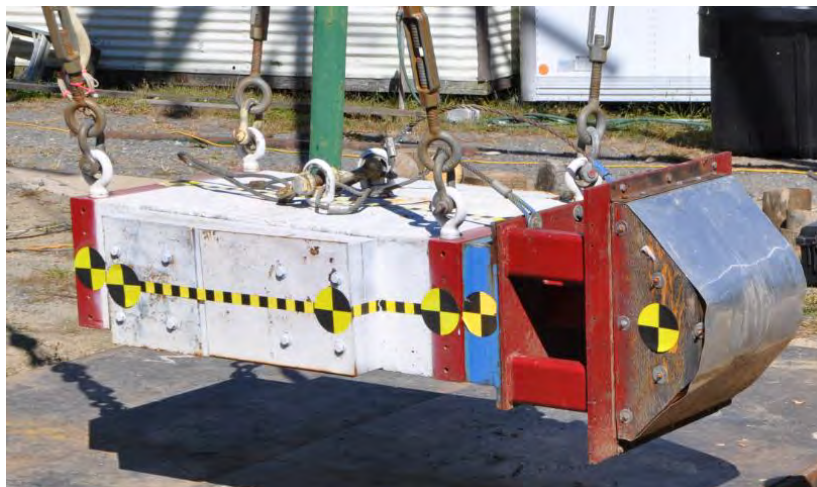
Figure 247. 2,372-lb pendulum device with semi-rigid nose.
