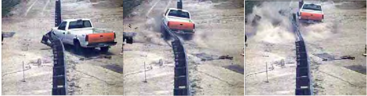
Figure 15. Test MGSDF-1 of the MGS guardrail with 7.25-inch diameter Douglas Fir posts. [Hascal07]
