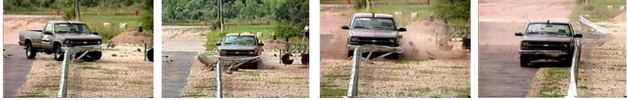
Figure 51. Sequential view of Report 350 Test 3-11 on the modified G2 at 32.25 inch rail height.[Buth00c]
