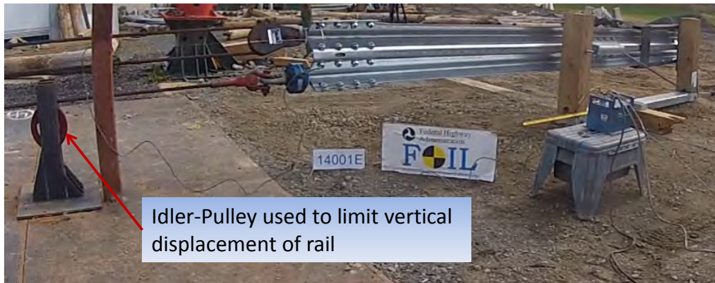
Figure 292. Idler-pulley mount used to maintain vertical position of loading cable.
