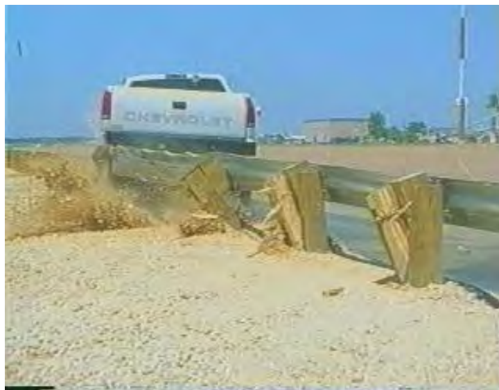
Figure 58. Guardrail damage in Test TTI 404201-1.[Bullard00]
