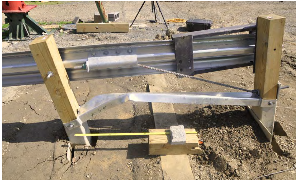
Figure 312. Post-test photo of Test 14001G for 8-inch reduced embedment case.
