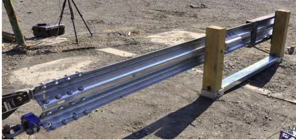
Figure 315. Pre-test photo of Test 14001H for 1" slack-cable case.
