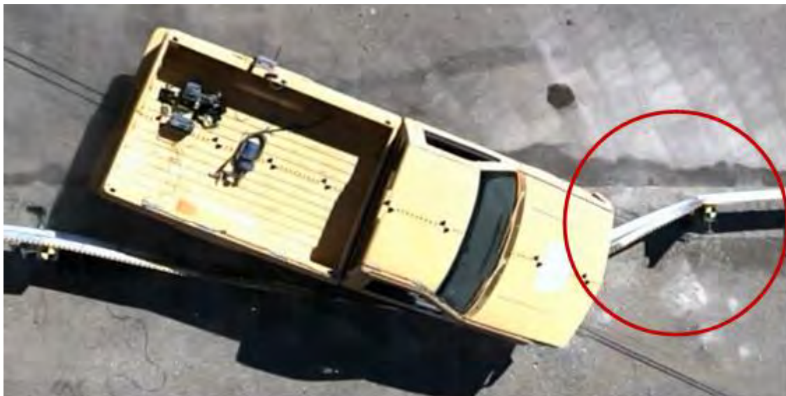
Figure 336. Pocketing during full-scale crash test C08C3-27.2.[Fleck08b]
