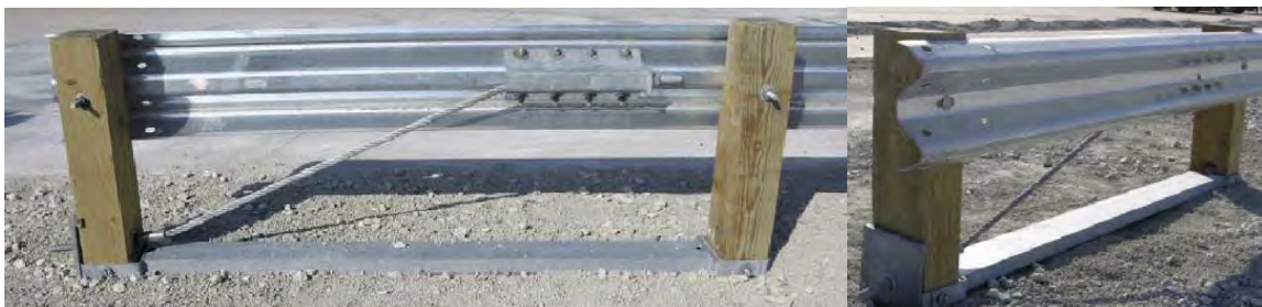
Figure 56. Generic end-terminal used in full-scale Crash Test 2214-WB1 of a strong-post guardrail system.[ Polivka06a ]
