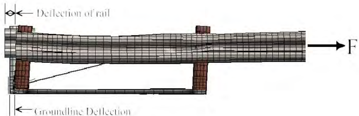
Figure 287. Example – finite element model for computing force-deflection response of the standard two-post guardrail anchor system.[Plaxico03]
