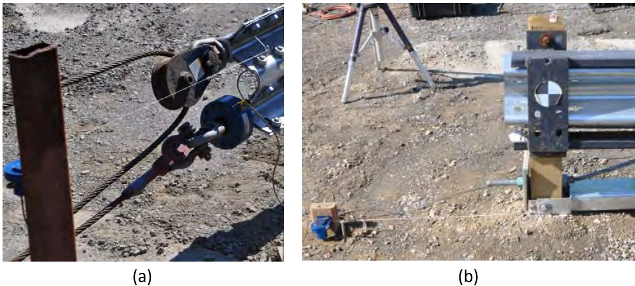
Figure 294. Displacement transducers mounted to (a) w-beam rail at load point and (b) top of foundation tube at Post 1.
