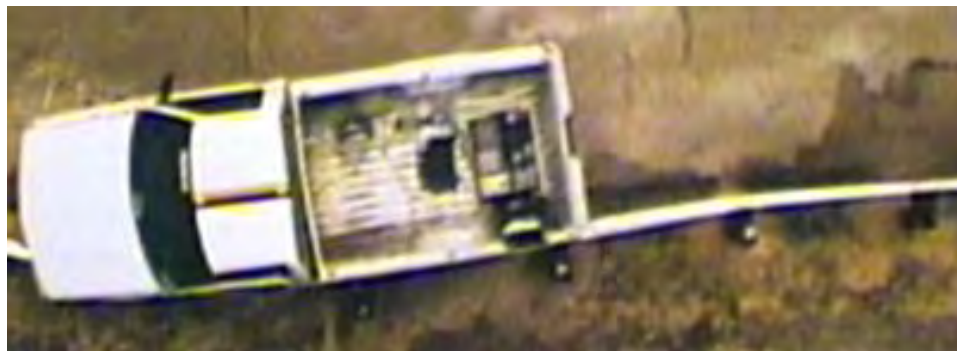
Figure 201. Snapshot from 471470-26 illustrating torsion behavior of posts upstream of impact on the G4(2W).[Mak99a]
