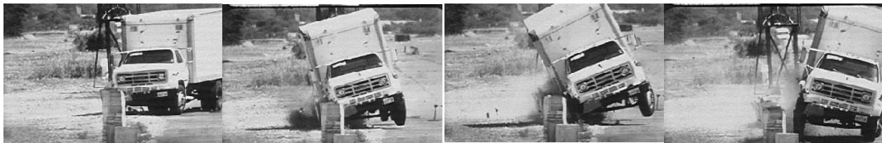
Figure 25. Sequential photos for Test 404211-5a on the modified three-beam guardrail under NCHRP Report 350 Test 4-12 conditions. [Buth99c]
