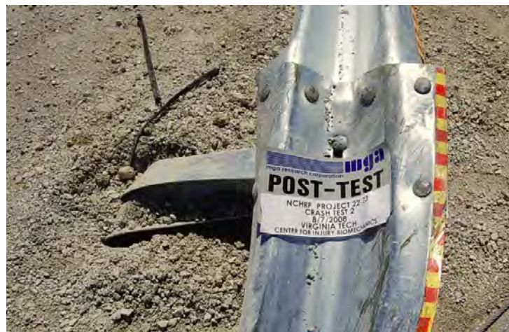
Figure 61. Post-test photo for Test MGA C08C3-027.2 showing the un-failed rail-post connection which resulted in the post pulling the rail down during impact.[ Fleck08b ]
