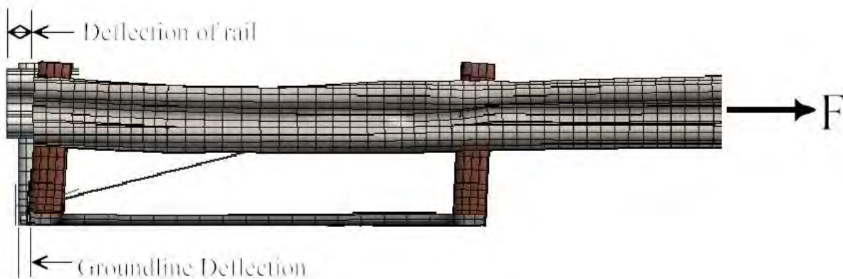
Figure 176. Example – finite element model for computing force-deflection response of the standard two-post guardrail anchor system.[Plaxico03]
