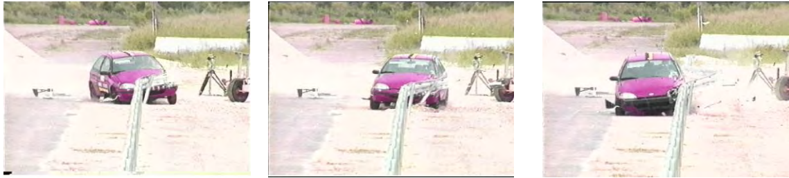
Figure 52. Sequential view of Report 350 Test 3-10 on the modified G2 at 32.25 inch rail height.[Buth00e]
