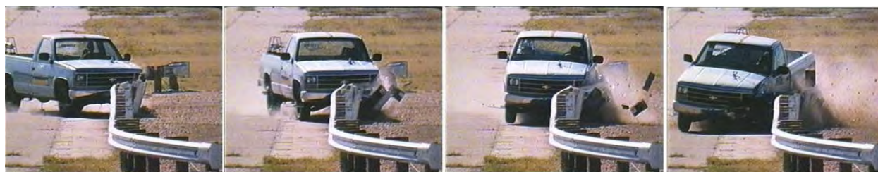
Figure 2. Sequential views of Crash Test 405421-1.[Bullard96]
