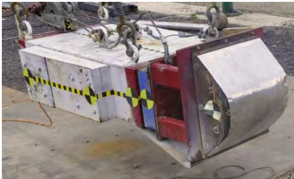
Figure 250. Repair to the pendulum head included adding a steel “slide Plate” underneath the head.
