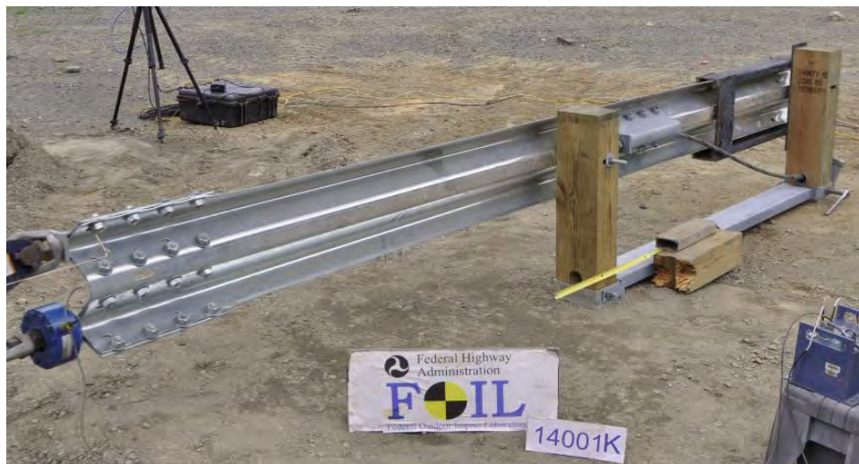
Figure 317. Pre-test photo of Test 14001K for 3” slack-cable case.
