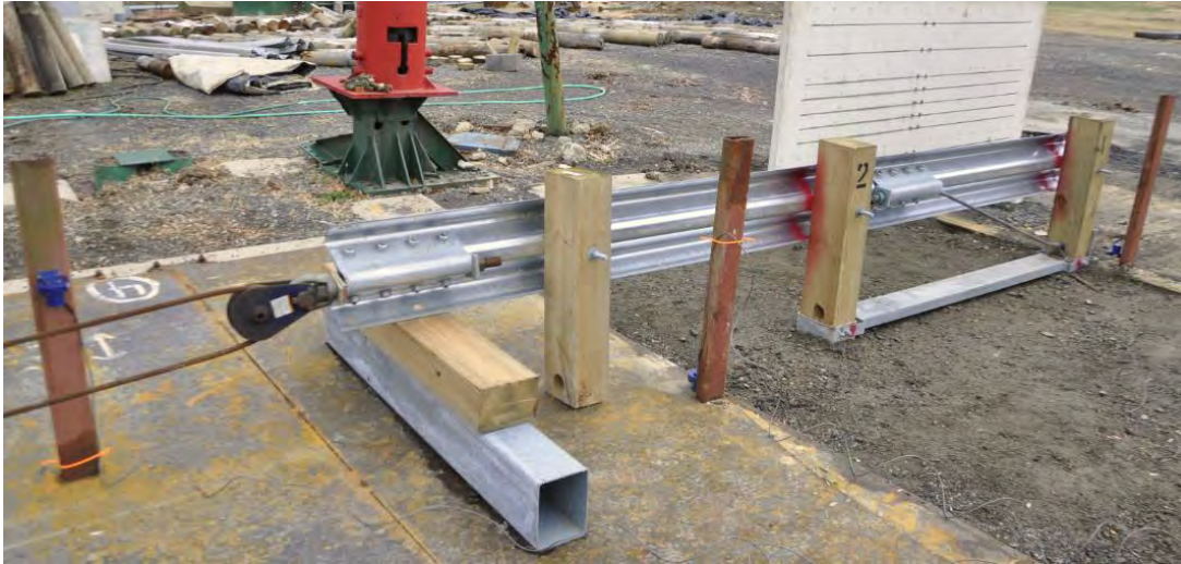
Figure 177. Test set-up for measuring force-deflection response of a standard two-post guardrail end-terminal anchor.
