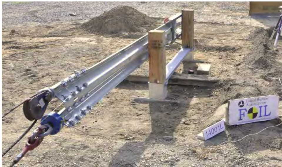
Figure 307. Pre-test photo of Test 14001L for 6-inch reduced embedment case.
