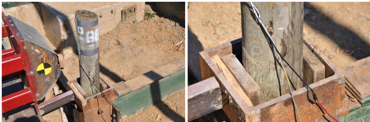
Figure 114. Rigid steel sleeve used for post mounting.
