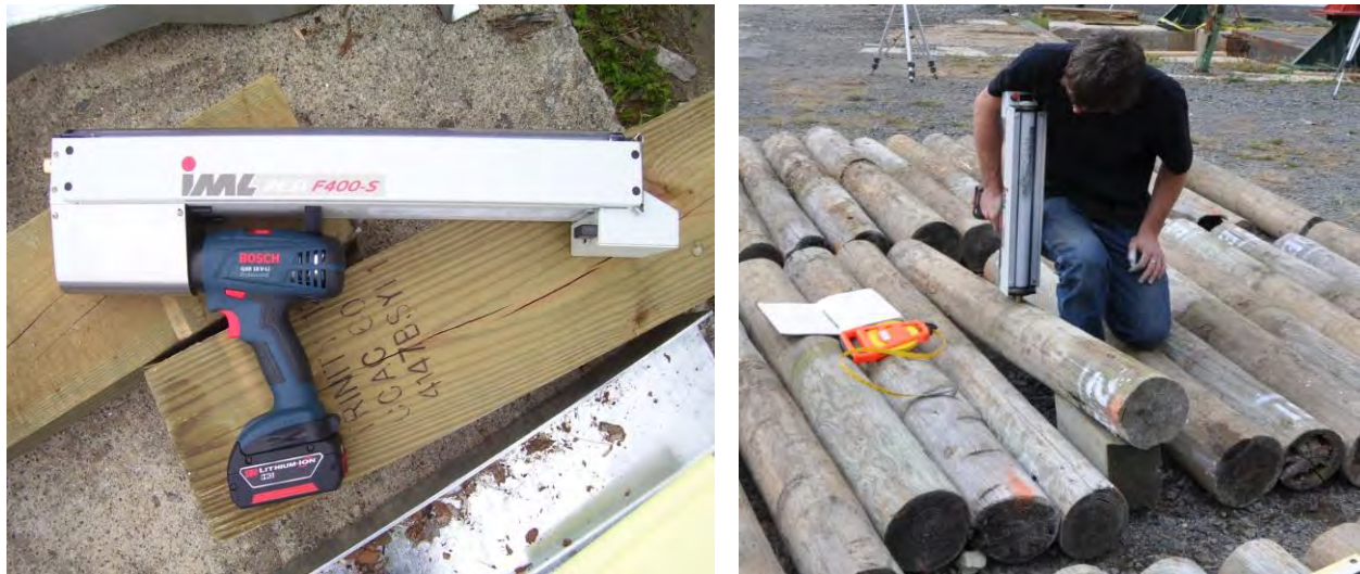
Figure 105. IML Resi-F400 S Resistograph.
