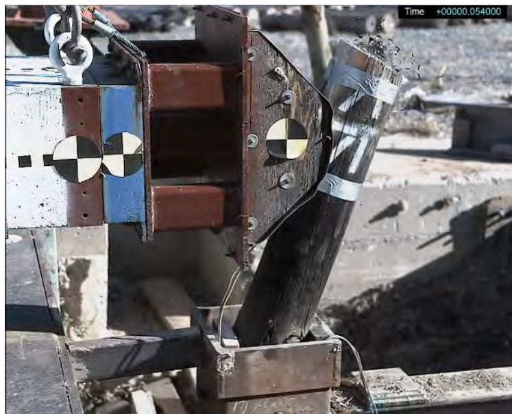
Figure 118. Photo of Test 13009G1 showing Post 71 breaking below groundline.
