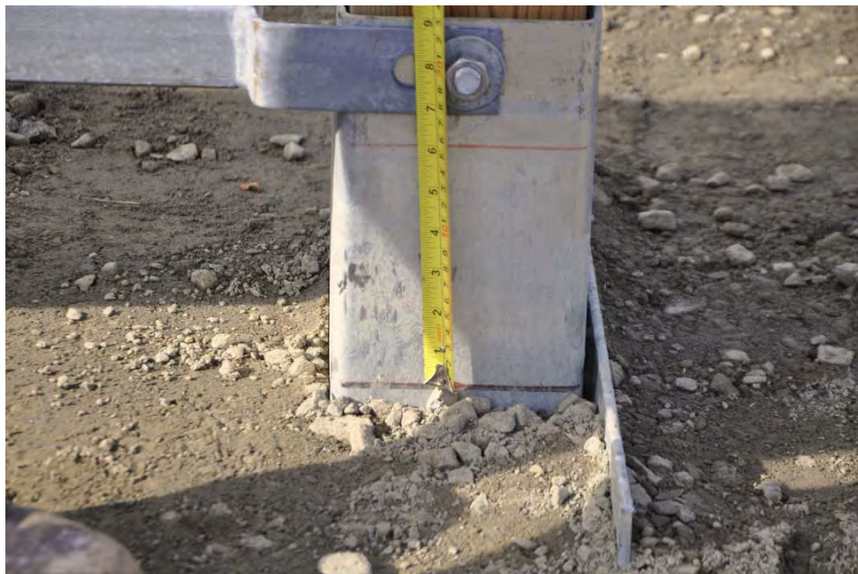
Figure 304. Procedure for measuring reduced embedment depth.
