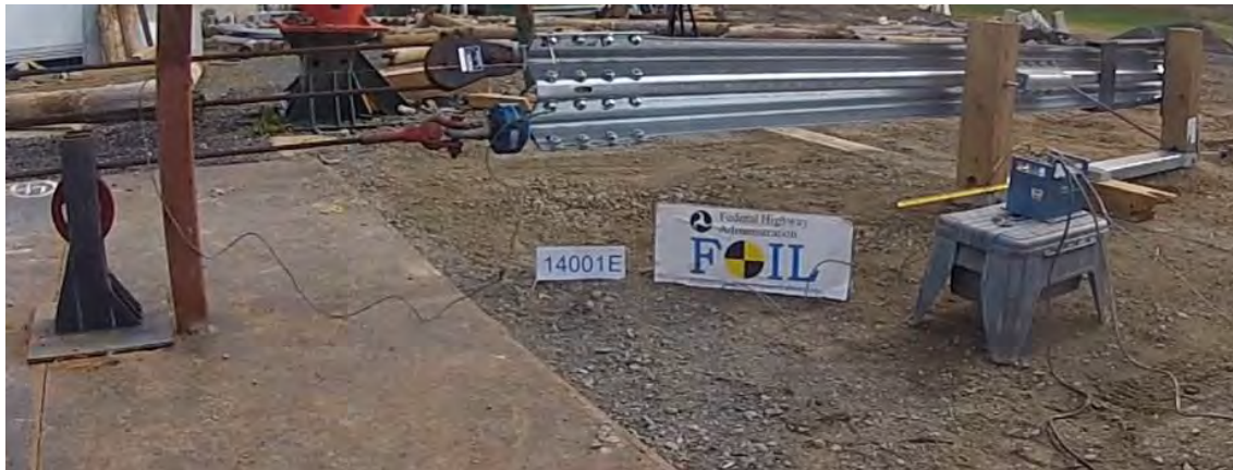
Figure 288. Typical test set-up for measuring force-deflection response of the guardrail end-terminal anchor.
