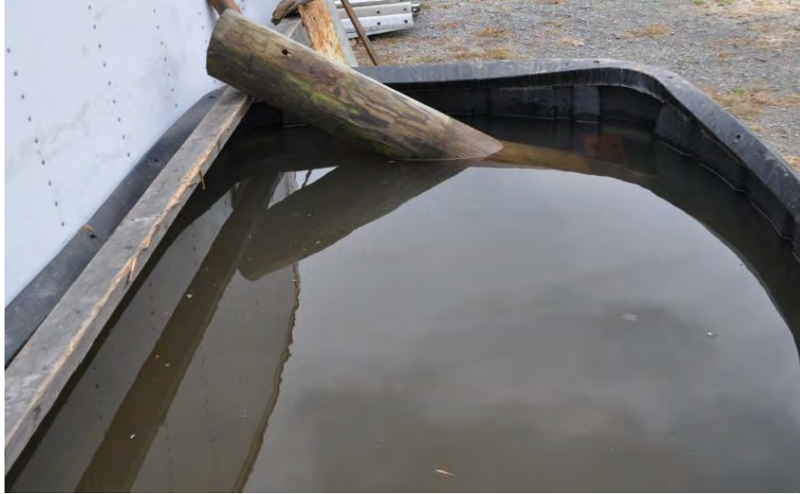
Figure 113. Photo of post specimen soaking in tank of water.
