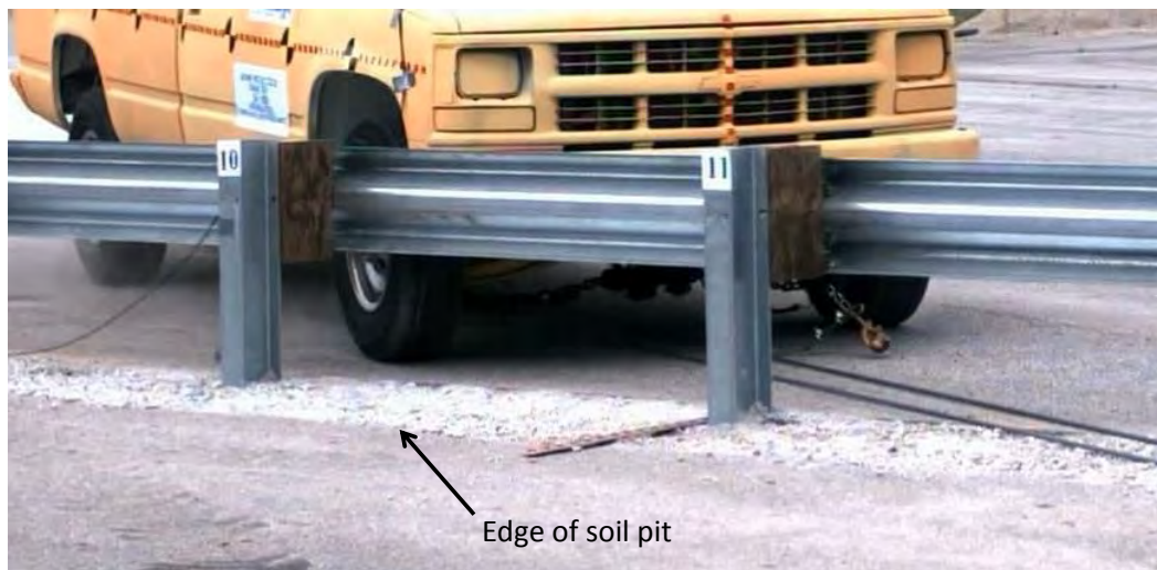
Figure 233. Test setup for low-speed test C08C3-027-1 illustrating the limited distance to the back-edge of the soil-pit for the test article.
