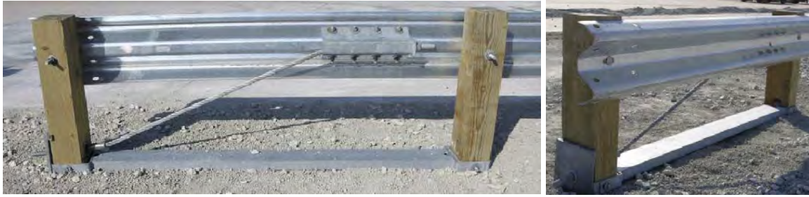
Figure 175. Generic end-terminal used in full-scale crash test 2214-WB1 of a strong-post guardrail system.[Polivka06a]
