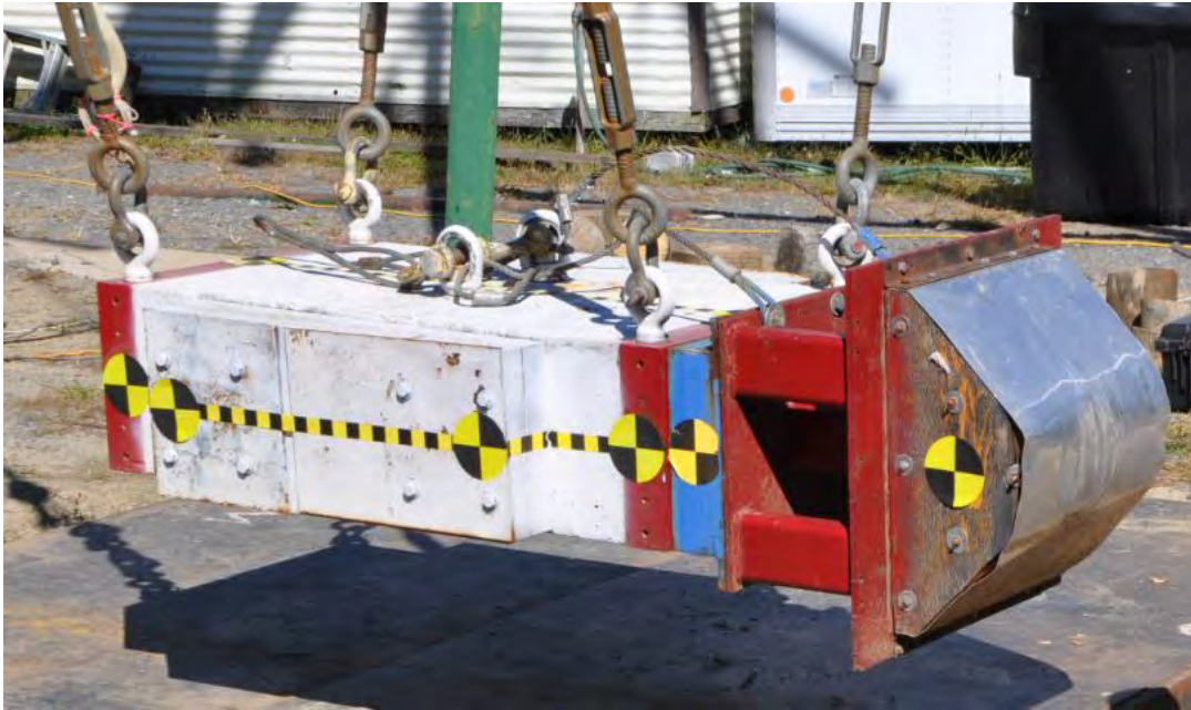
Figure 115. 2,372-lb pendulum device with semi-rigid nose.
