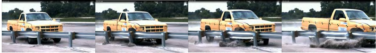
Figure 27. Low-speed Test C08C3-027.1 on the modified G4(1S) with routed wood blockouts. [Fleck08]
