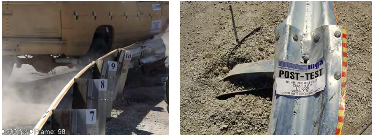
Figure 213. Results of Test MGA C08C3-027.2 illustrating torsional deformation of the W6x8 steel guardrail posts during vehicle collision.[Fleck08b]
