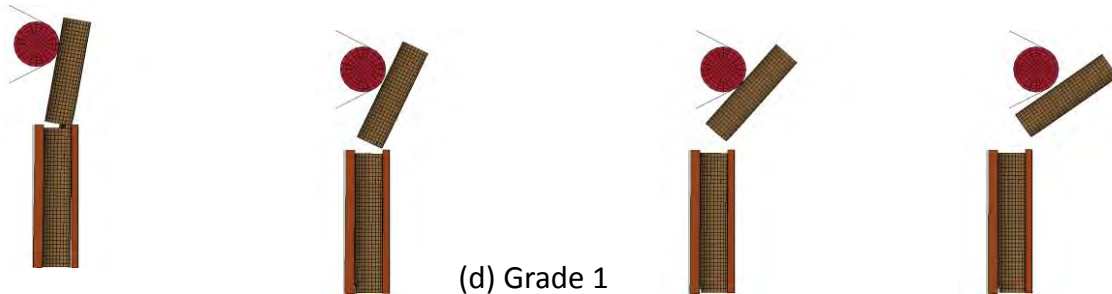
Figure 82. Sequential views of (a) Test 13009L and analyses for post model with pre-defined MAT143 properties for (b) clear wood, (c) grade DS-65 and (d) grade 1.
