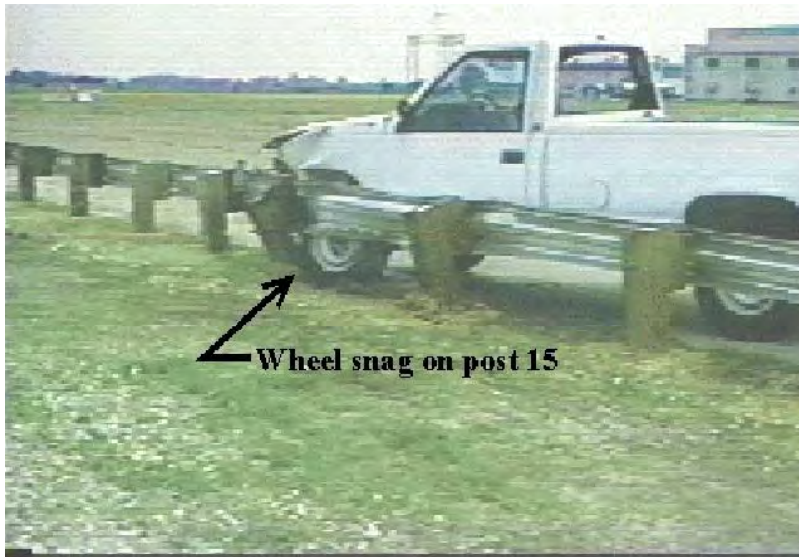
Figure 39. Wheel snag against guardrail post in TTI Test 471470-26.[Mak94]
