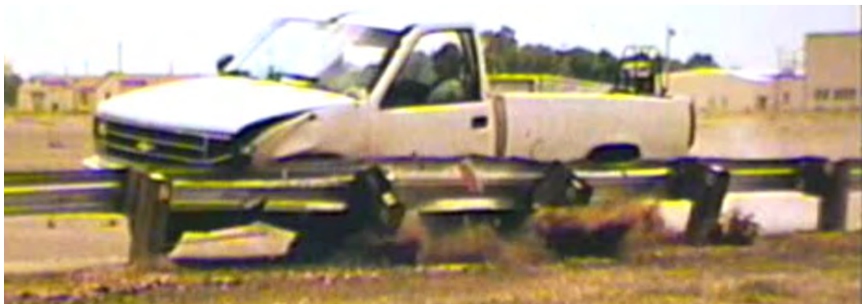
Figure 214. Results of Test 471470-26 illustrating the response of the wooden guardrail posts during vehicle collision.[Mak99]
