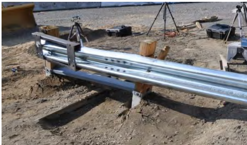
Figure 311. Post-test photo of Test 14001L for 6-inch reduced embedment case.
