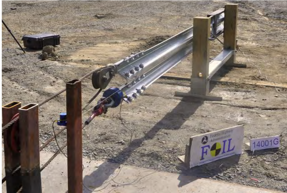
Figure 308. Pre-test photo of Test 14001G for 8-inch reduced embedment case.
