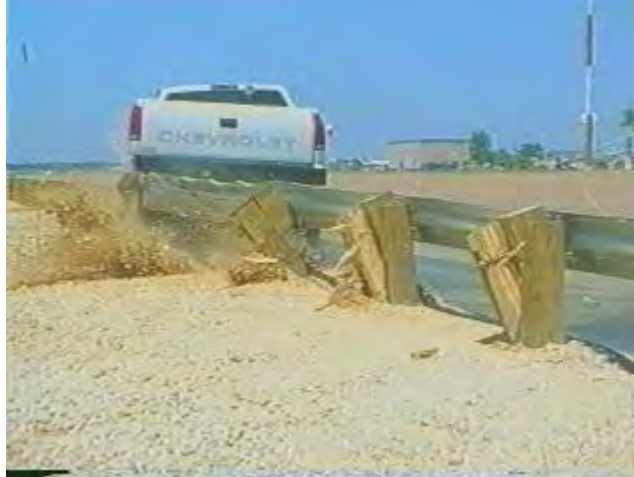
Figure 215. Results of Test 404201-1 illustrating brittle fracture of wood posts due to tensile forces in the w-beam rail.[Bullard00]
