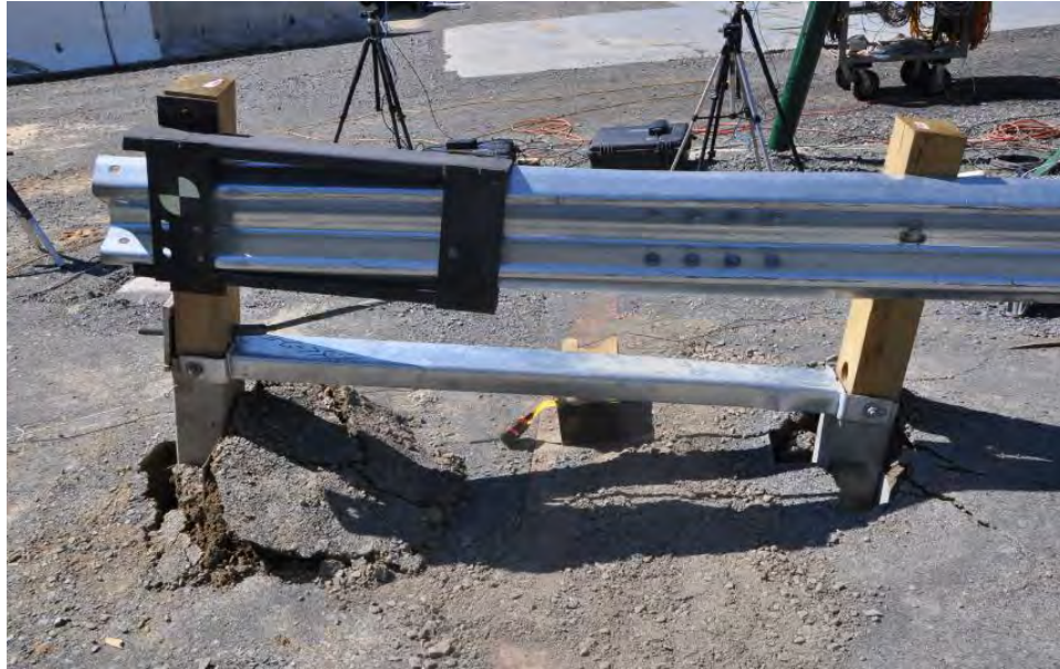
Figure 310. Post-test photo of Test 14001F for 4-inch reduced embedment case.
