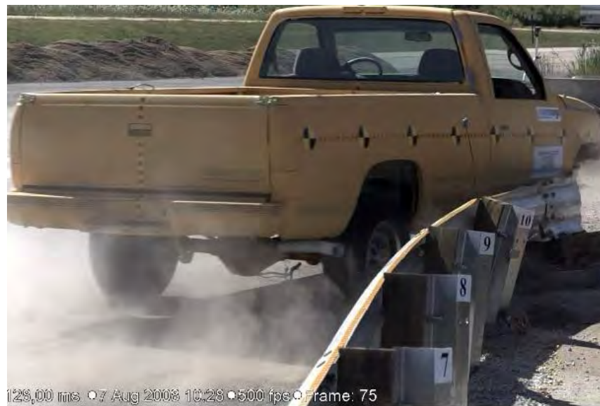
Figure 200. Snapshot from Test C08C3-2 illustrating torsion behavior of posts upstream of impact on the G4(1S).[Fleck08b]
