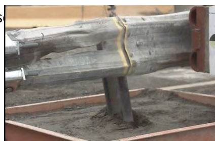
Test 14004I (rail tear at left boundary)
