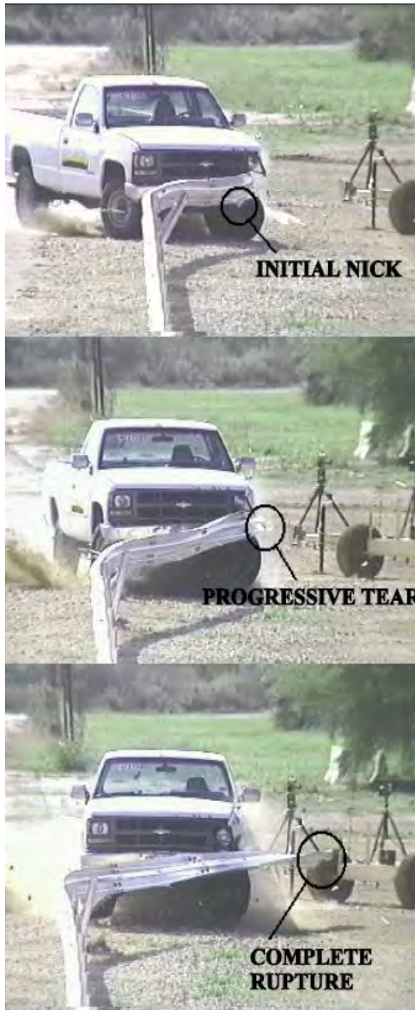
Figure 50. Test 473750-1 on a weak-post w-beam guardrail resulting in rail rupture. [Buth00a]
