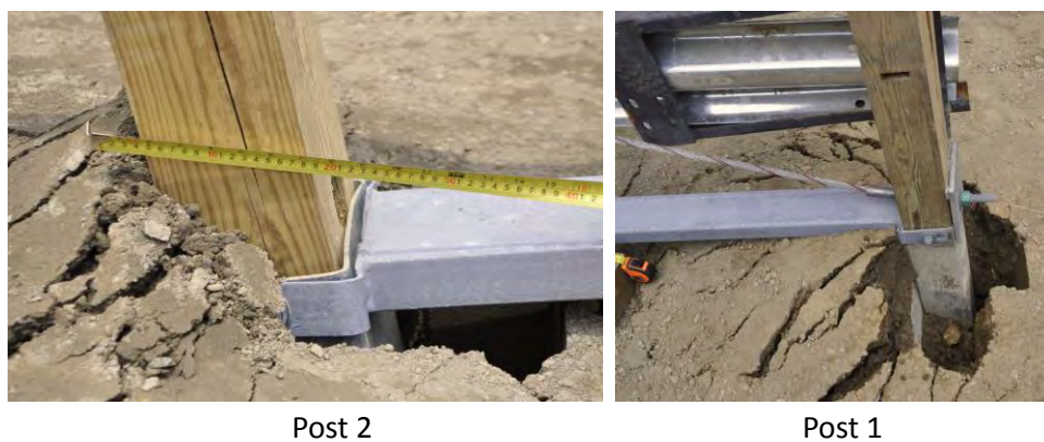
Figure 321. Post-test photos of Test 14001K for 3” slack-cable case.
