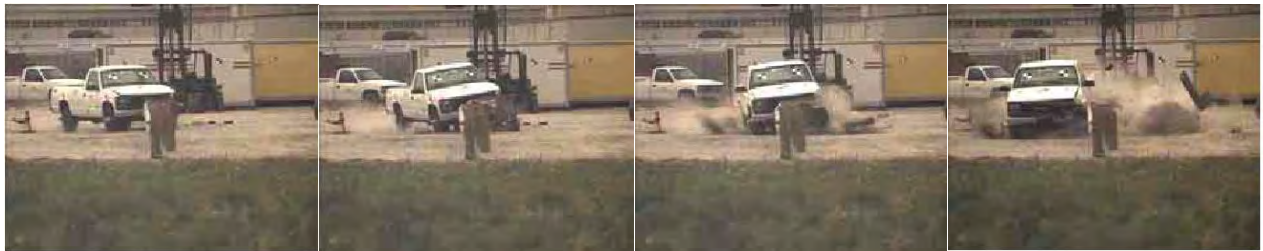
Figure 16. Test MGSPP-1 of MGS with 8-inch diameter Ponderosa Pine posts. [Hascal07]
