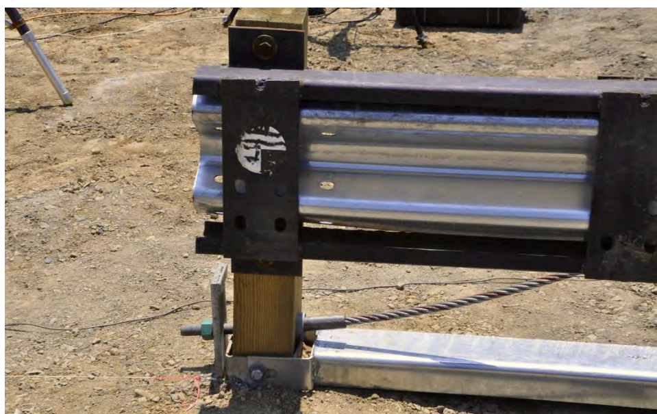
Figure 318. Pre-test photo of Test 4001J for 4” slack-cable case.
