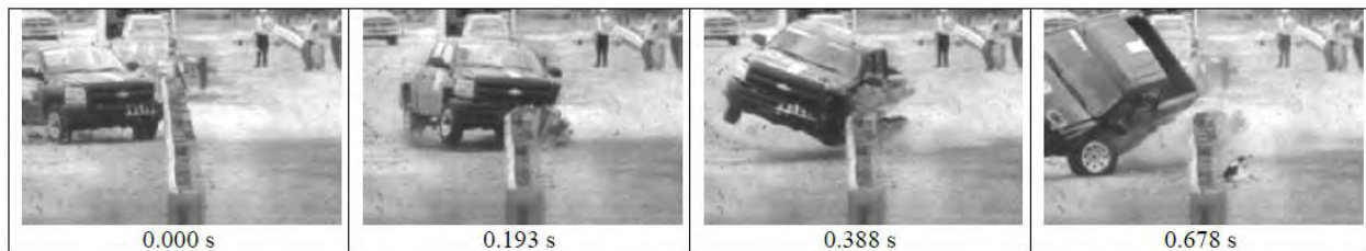
Figure 22. Sequential photos for Test 476460-1-8 on the thrie-beam guardrail with routed wood blockouts (MASH Test 3-11).[ Bullard10 ]
