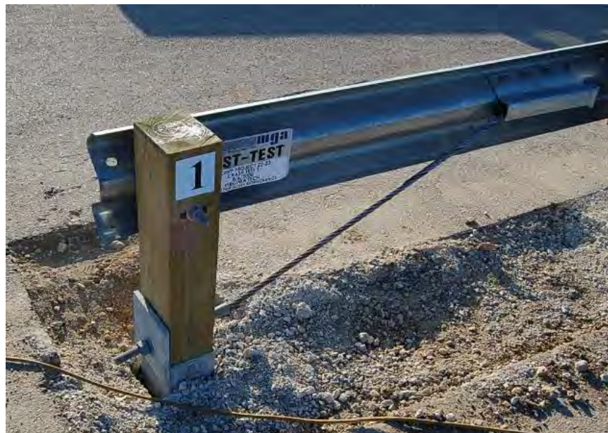
Figure 223. Photo of upstream anchor after Test C08C3-027-1. [Fleck08a]
