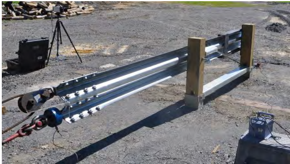
Figure 306. Pre-test photo of Test 14001F for 4-inch reduced embedment case.
