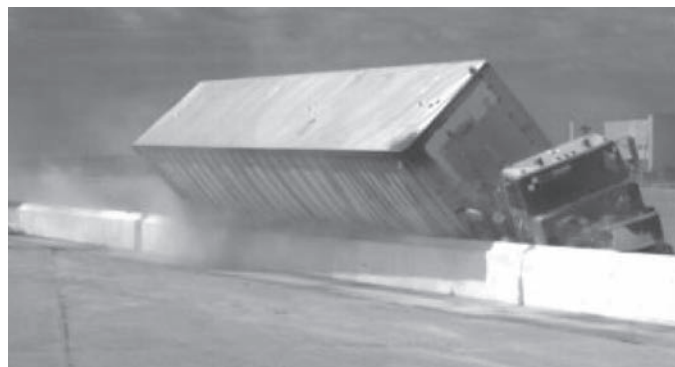
Figure 24. Tractor-trailer truck leaning over a 42-in.-tall concrete barrier [Rosenbaugh 2007].
