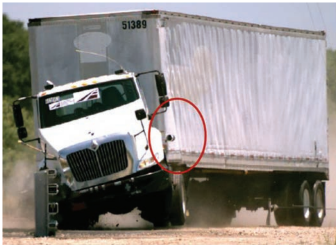
(a) Trailer rupture
