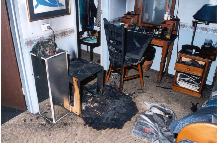
Figure 3. Locally under-ventilated fire in a nightstand resulting in one fatality. Photo courtesy of Ross Brogan AFSM, MA, IAAI/CFI, GWBFORENSIC, NSW, Australia.
