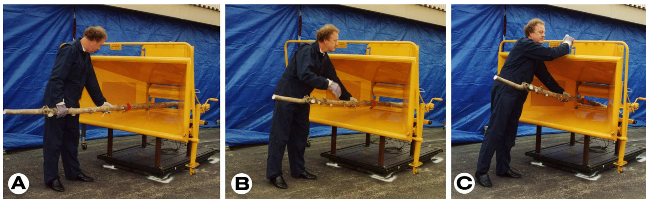
Figure 3. Test Subject 7, Left Hand Attached to Branch, Center Feed Hopper Position
